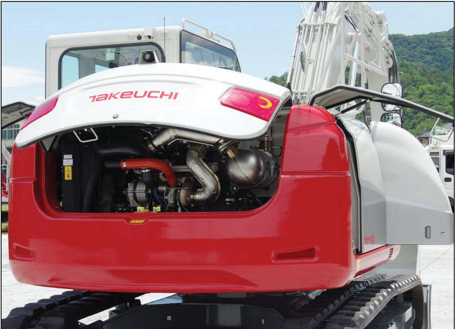
Large lockable service hood provide vandalism protection and outstanding maintenance access.
